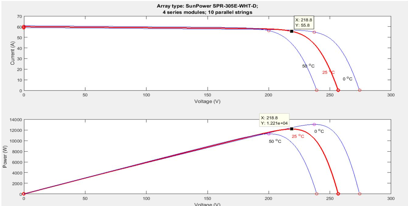
Fig. 4 PV and IV curves of the PV system
