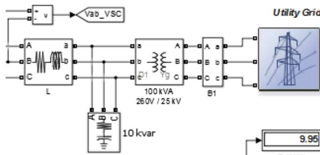
Fig. 3: Filter and capacitor bank for smooth curves
