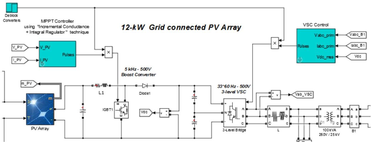
Fig. 2: VSC control of for the inverter
