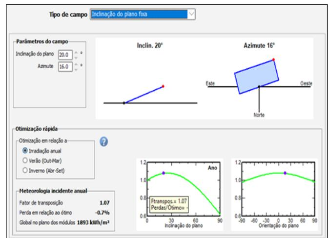
Figure 3. Setting the orientation of the photovoltaic system.
