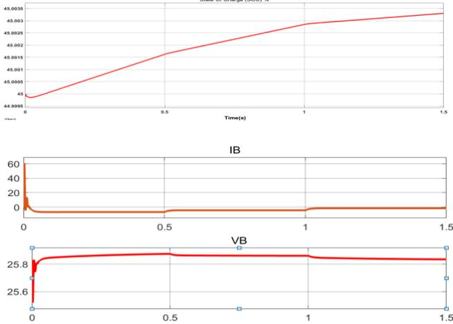
**Fig 18.** Battery Performnce : SOC , Cuurent and Voltage.
