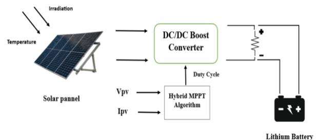
Fig 1 .Configuration of the PV system
