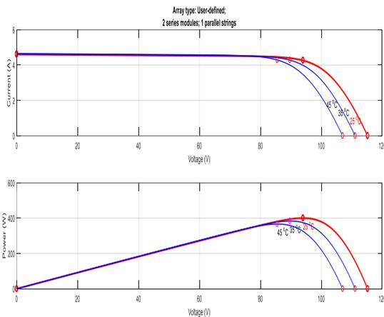
Fig 3 .I-V and P-V characteristics under fixed irradiance and variable temperature
