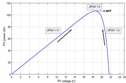
Fig 5. P-V curve for (P&O) algorithm
