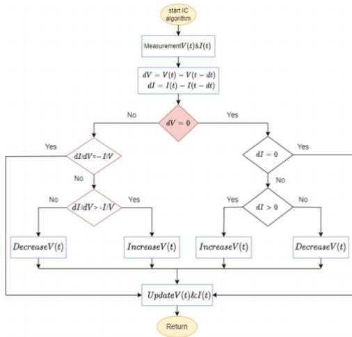
Fig 6. Flowchart of INC algorithm
