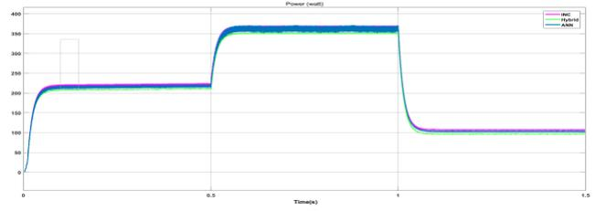
**Fig 12.** Load power with INC, ANN under variable irradiation conditions
