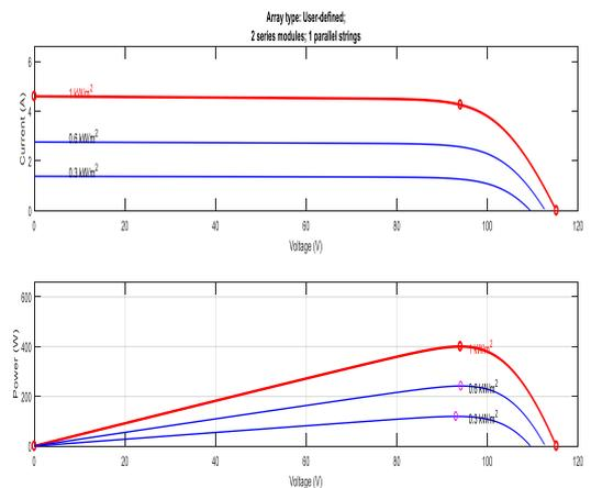
Fig 4 .I-V and P-V Curve under fixed temperature and variable irradiance
