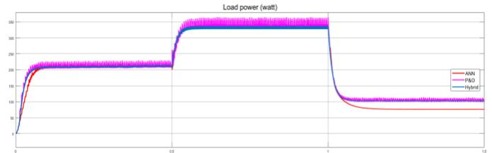
**Fig 13.** Load power Hybrid P&O,ANN, in under variable irradiation conditions
