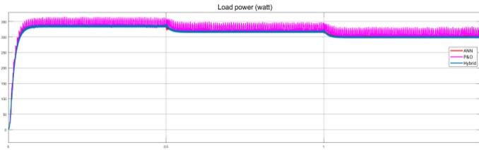
**Fig 17.** Load power under Hybrid algorithm of ANN, P&O under variable temperature conditions
