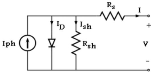
Fig 2 .PV Cell schematic circuit
