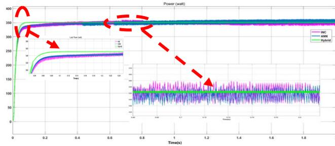
**Fig 9.** Load power under Hybridation of INC,ANN, in optimal solar conditions
