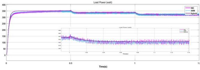
**Fig 16 .** power under Hybrid algorithm of ANN,INC under variable temperature conditions.
